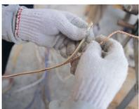
Shen Zheng-yi (沈正宜): Although the stripper is well designed and built, it still takes time and practice to operate proficiently. You need to maintain just the right amount of tension between the cutting edge and the surface of the wire: not too tight and not too loose. If you set the tension too tight, the handle is too hard to crank and the cutting edge wears down too quickly. If you set the tension too low, you can't slice open a fissure deep enough to separate the coating from the metal core.
